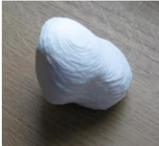
Fig. 6. The bladder physical model made of ABS using the FDM method Source: own study
