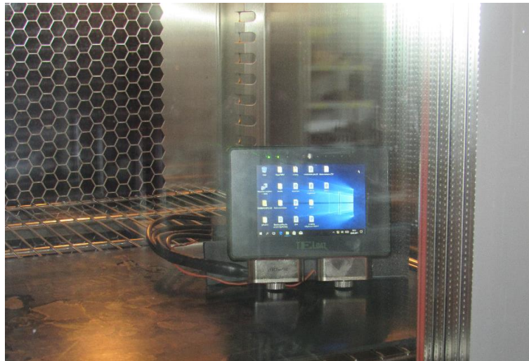
Fig. 5. Testing of the Tablet 3 model on the impact of high humidity in a climatic chamber Source: own photo
