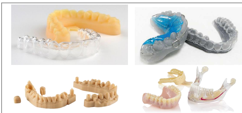
Fig. 9. Application of 3D printing in dentistry and prosthodontics – prostheses made by PolyJet and DLP Source: own study based on: [11-13, 21, 28, 32]
