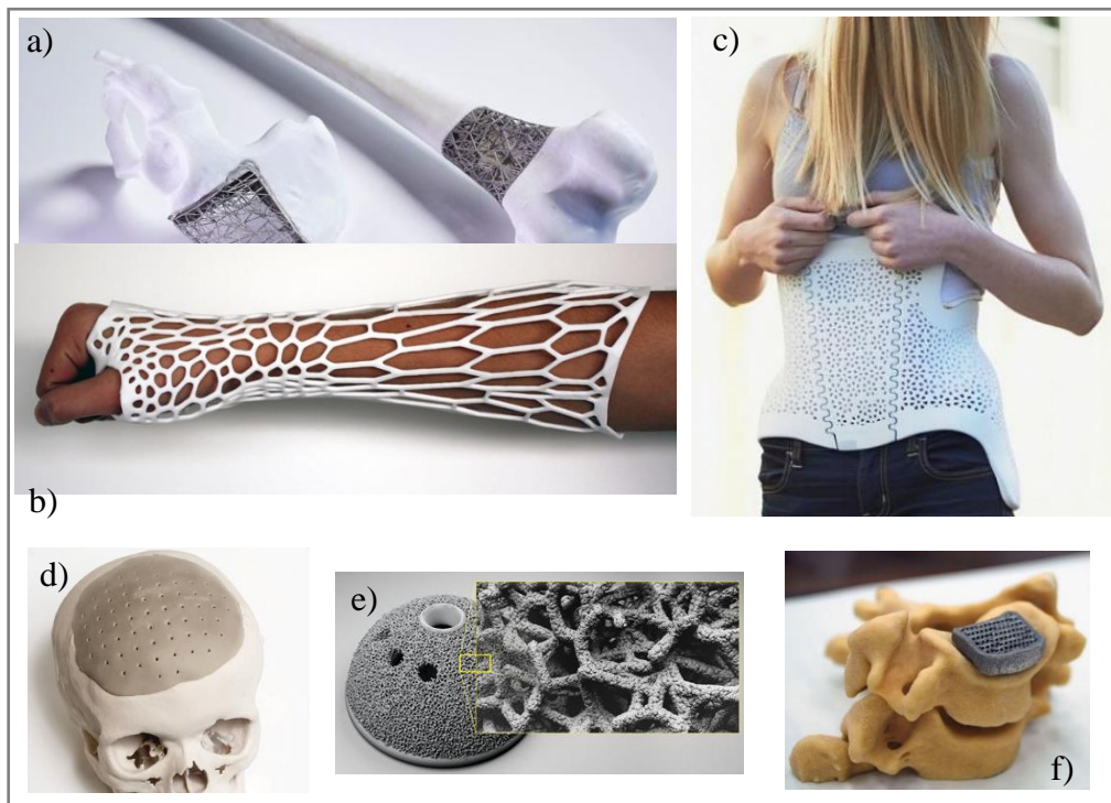
Fig. 5. Examples of application of 3D printing in surgery and orthopedics – elements filling bone cavities (a), Cortex replacing accustomed cast (b), Bespoke back brace made-up by SLS method (c), implant of cranium bones (d), hip joint implant made by DMLS method (e) and intervertebral disc implant (f)
