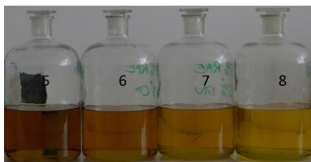
Fig. 3. ON and RME samples used for testing 5-RME, 6-50% RME + 50% ON, 7-20% RME + 80% ON, 8-ON Source: Own picture
