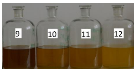
Fig. 4. ON and RME samples used for testing 9-RME + 2% water, 10-50% RME + 50% ON + 2% water, 11-20% RME + 80% ON + 2% water, 12- ON + 2% water Source: Own picture
