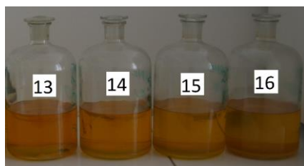
Fig. 5. ON and RME samples used for testing 13-RME + 2% water + light, 14-50% RME + 50% ON + 2% water + light, 15-20% RME + 80% ON + 2% water + light, 16-ON + 2% water + light Source: Own picture
