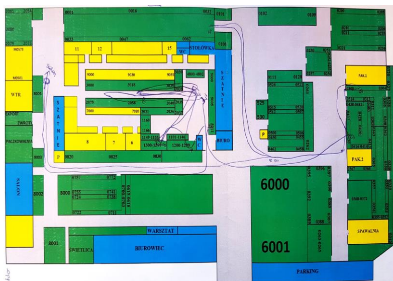
Fig. 4. Analysis of individual orders made using the spaghetti method
