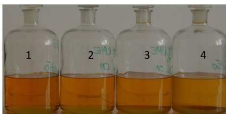
Fig. 2. ON and RME samples used for testing 1-RME + light, 2-50% RME + 50% ON + light, 3-20% RME + 80% ON + light, 4-ON + light Source: Own picture
