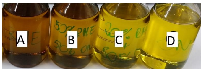
Fig. 1. Fresh samples ON and RME used for testing A-RME fresh, B-50% RME + 50% ON fresh, C-20% RME + 80% ON fresh, D-ON fresh Source: Own picture
