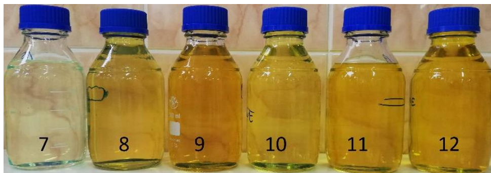
Fig. 3. Diesel and RME samples aged for 16 weeks
