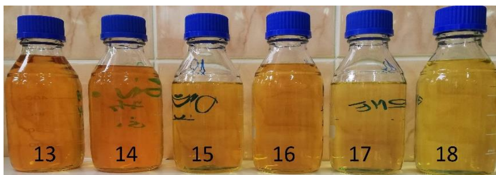
Fig. 4 The appearance of samples aged with the action of light and the content of 2% water
