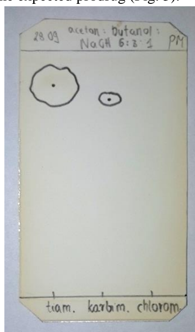
Fig. 5. TLC plate for acetone:butanol:sodium hydroxide (10%) phase (6:3:1) Source: own development
