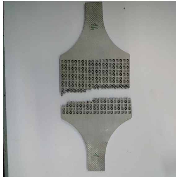
Fig. 2. Example of an aluminum lattice structure plate broken after tensile test Source: own work
