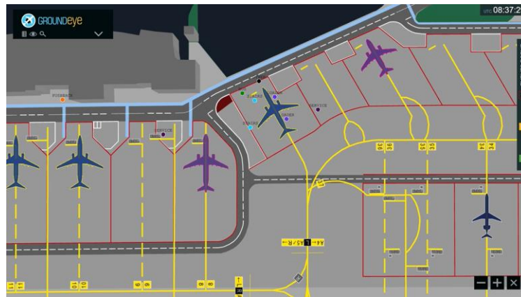
Fig. 4. A application frontend screen showing the positions of aircrafts and tracked assets in a typical operations mode Source: own work
