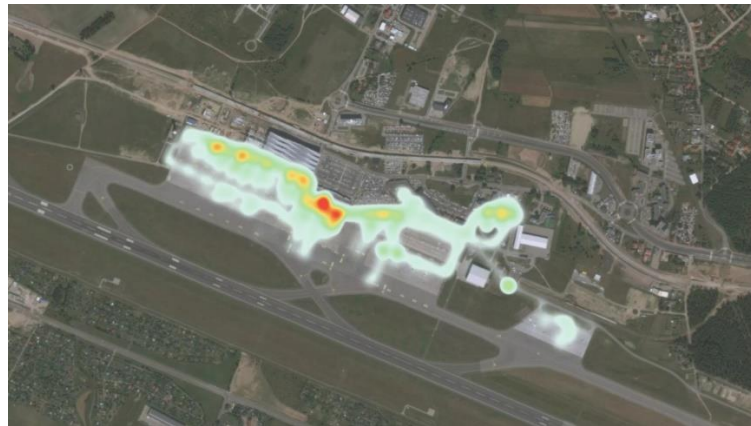
Fig. 1. A composite image containing all tracked data presented on a map of airport, colour represents how often assets have been detected in the area (red – most often)
